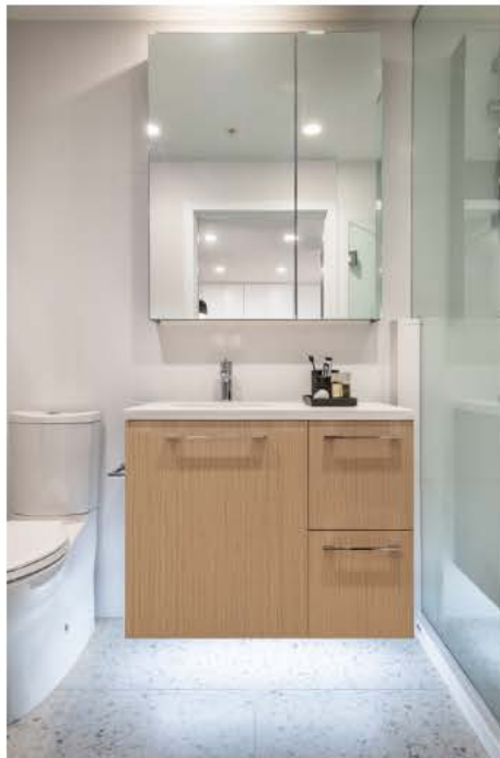
Floating vanity with under-cabinet motion sensor lighting complete with soft-close hardware
